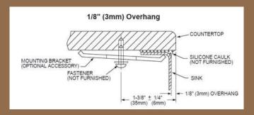
Electronic Template Mounting Option (Download DXF File from www.msisurfaces.com) NOTE: THIS UNDERMOUNT SINK IS DESIGNED TO MOUNT TO SOLID SURFACE (NON-LAMINATE) COUNTERTOP ONLY.
