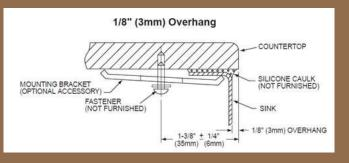
Electronic Template Mounting Option (Download DXF File from www.msisurfaces.com) NOTE: THIS UNDERMOUNT SINK IS DESIGNED TO MOUNT TO SOLID SURFACE (NON-LAMINATE) COUNTERTOP ONLY.
