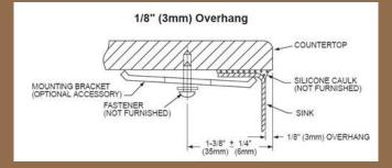
Electronic Template Mounting Option (Download DXF File from www.msisurfaces.com) NOTE: THIS UNDERMOUNT SINK IS DESIGNED TO MOUNT TO SOLID SURFACE (NON-LAMINATE) COUNTERTOP ONLY.
