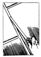
**3.** Apply mix to joints with a grout floar making certain joint is completely filled with mix.
