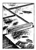
**4.** Maintain a grout space between the pieces as recommended by the slate supplier (1/4" or 3/8") depending on the sizes of the tiles. To do these accuretaly, use spacers. Slate may also be laid without joints, in which case edges are then butted against one another, only if the Material is honed or polished, however we recommend 1/16" - 1/8" grout joint.
