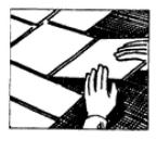
3. Using a notched 1/4" x 1/4" trowel, hold at a 45 degree angle to be sure a full ridge is made with the notches. Spread thinset on floor starting ar a far corner so you can back out of the room as you proceed. Spread just enough area so you can reach over it to place the slate.
