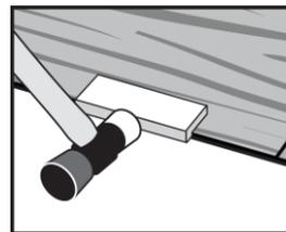
**Note:** When starting a new row, you can use the cut piece from the previous row, as long as it is more than 8" (20.3cm) and the stagger between seams still is greater than 8" (20.3cm).
